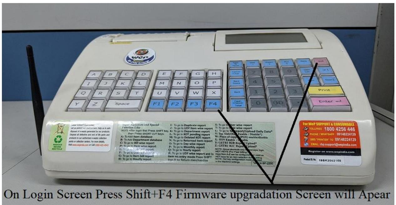
On Login Screen Press Shift+F4 Firmware upgradation Screen will Appear
